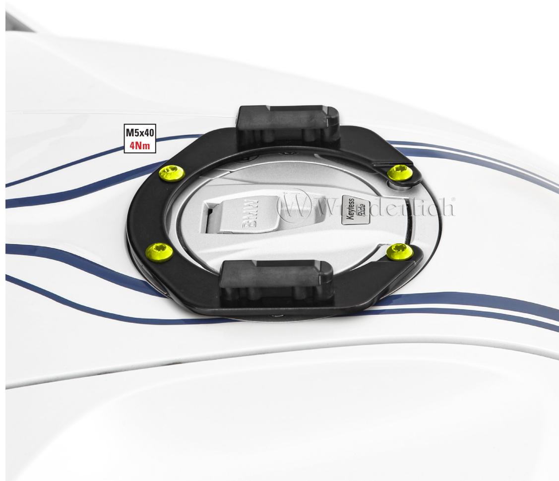
**NACH DER MONTAGE DES TANKRINGES, FUNKTION DES TANKDECKELS PRÜFEN.
